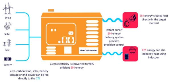
Acceleware's patented CTI heating 'engine' can provide intelligent, reliable, scalable, on-demand, decarbonized heat via EM energy. EM Powered Heat with CTI can be adapted to multiple industrial clean heating applications, displacing fossil heating systems that are GHG intensive and costly to operate.
